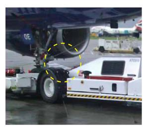
The investigation determined that a maintenance error had led to the fan cowl doors on both engines being left unlatched following scheduled overnight maintenance on the aircraft (pictures above). The unlatched condition of the fan cowl doors was not identified prior to the aircraft's departure the next
